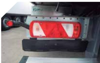
REF. 840501221 PILOTO ASPOCK ECOLED C/CUERNO DERECHO ECOLED REAR RIGHT SIDE LIGHT WITH GALIBO LIGHT
