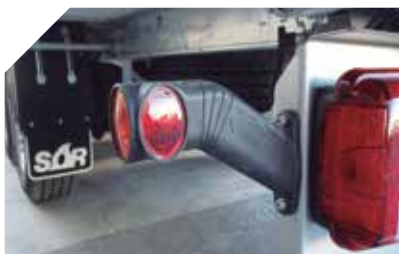
REF. 840501222 PILOTO GALIBO VIGNAL CUERNO CURVO LED "IZQUIERDO" LEFT SIDE STANDARD GALIBO LIGHT
