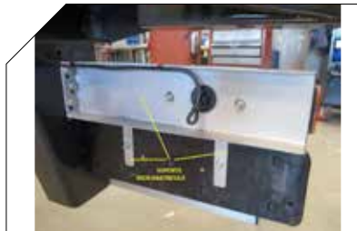
REF. 366501203 SOPORTE INOX CHAPA INOX PILOTO +MATRICULA ST ST REAR CHAMBER LIGHT ST ST PLATE SUPPORT REGISTER PLATE LIGHT
