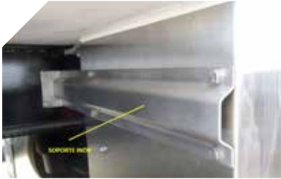
REF. 366500100 SOPORTE GUARDABARRO INOX R-SENCILLA (OP) ST ST SINGLE WHEEL MUDGUARD SUPPORT
